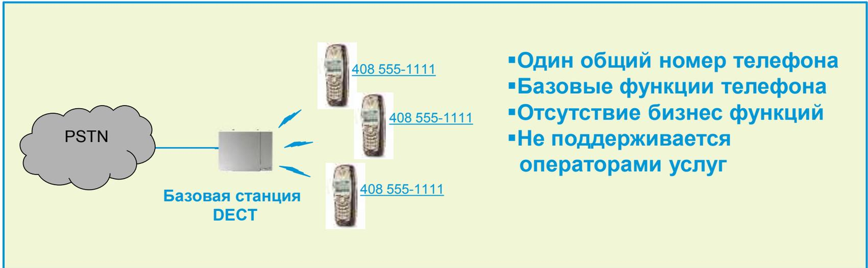
The diagram illustrates a Consumer DECT system. On the left, a cloud labeled 'PSTN' is connected to a central 'Базовая станция DECT' (DECT Base Station). Three mobile phones are shown to the right of the base station, each with the number '408 555-1111' displayed next to it. Blue arrows point from the base station to each phone.
